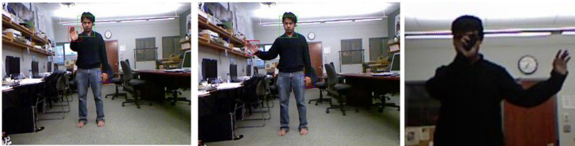
Fig. 4. Although a user's hand can be localized by hand tracking algorithms (left & middle), there are factors, e.g. , lighting condition and neighborhood color; that can make it temporarily disappear. With a mobile in hand (right), localization is reduced to device tracking, which is easier due to the distinct outline and color.
